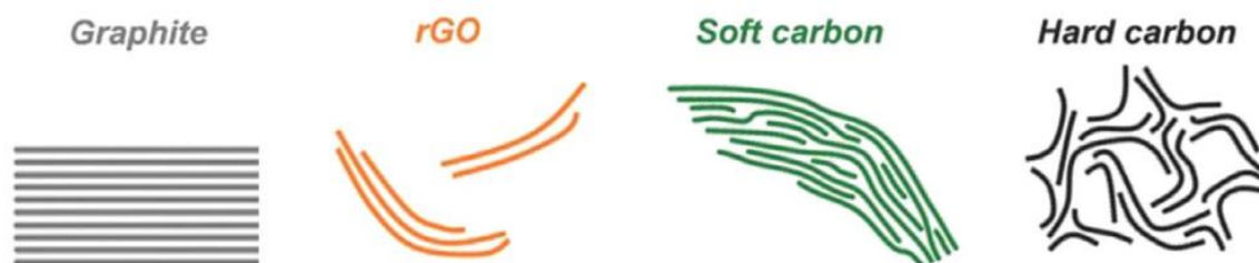
Figure I.7. Scheme of the structure of various carbonaceous materials [48] .
