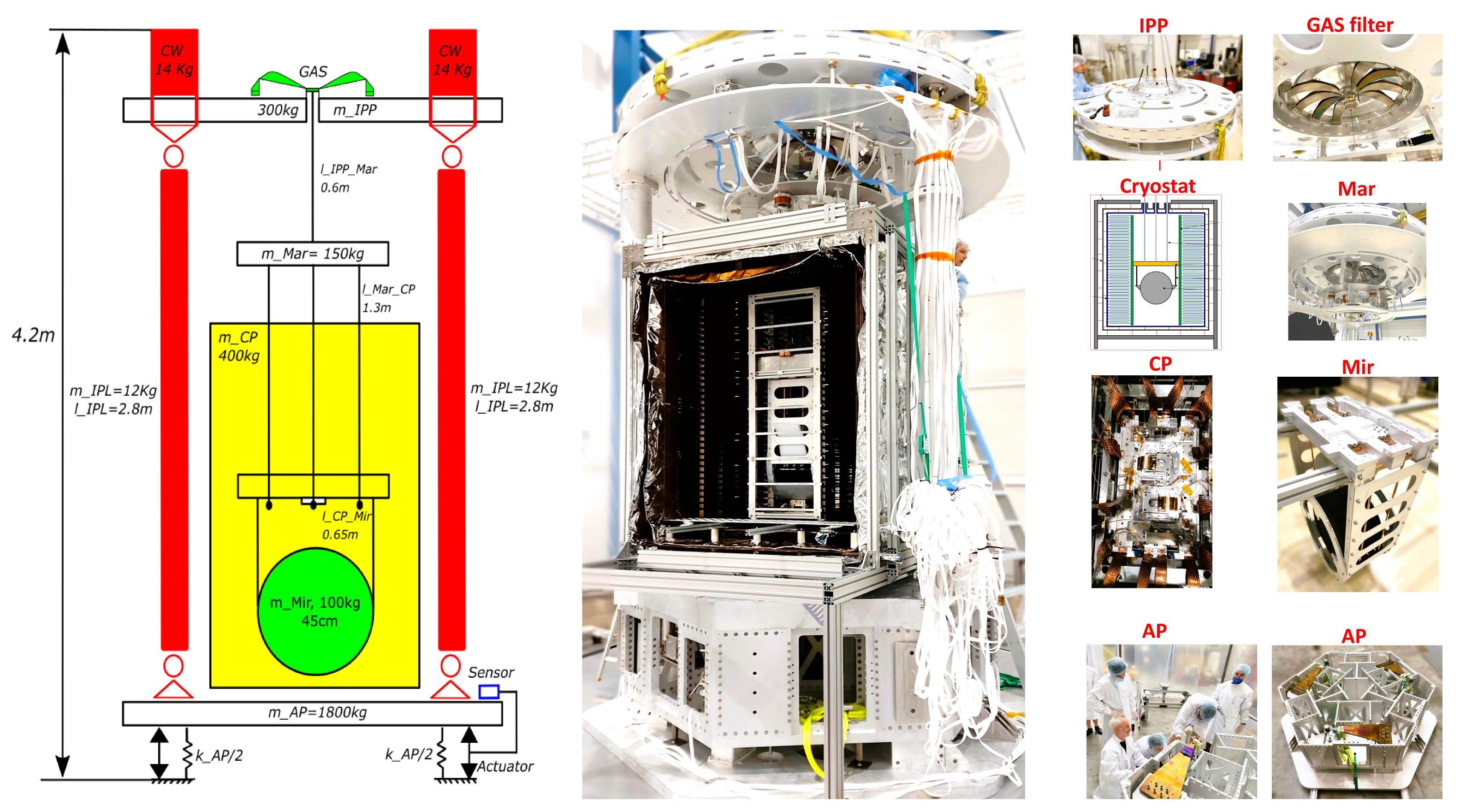
Abbreviation: AP: Active Inertial Platform, GAS: Geometric Anti-Spring, IPL: Inverted Pendulum Leg, IPP: Inverted Pendulum Platform, Mar: Marionette, CP: Cryostat+Cold Platform, Mir: Mirror, k: Stiffness, m: Mass, CW: Counter Weight
