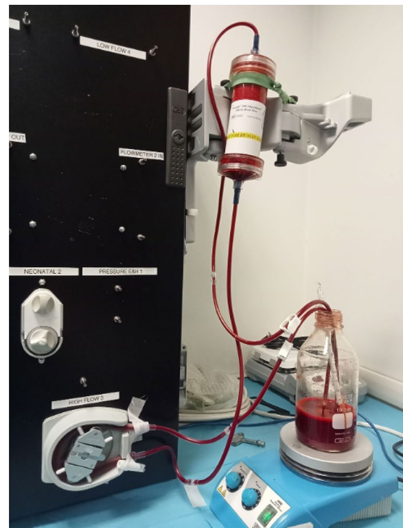
Fig. 1 (abstract 000292) Extracorporeal therapy in the treatment of sepsis: in vitro assessment of the effect of an absorbent cartridges on the circulating bacterial concentration (2 h of hemoperfusion)
