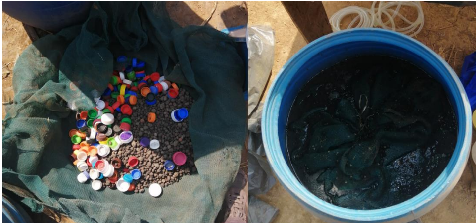
Figure 5-3. Preparation of aerobic biofilters (biomedica, plastic plugs and clay ball).
