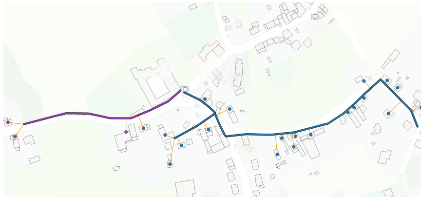
Figure 6.2: Considered network which consist of a subpart of the reconstructed Belgian network that have one single substation connected to two-feeders.
