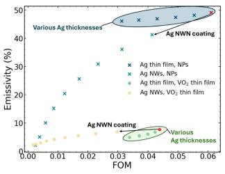
Fig. 4 Impact on the emissivity of varying the Ag thickness vs. the impact of adding Ag NW networks with various densities. In the case of the NP stack, adding a Ag NW network yields lower  $\ensuremath{\varepsilon}$  for a given FOM, making this addition positive. In the case of the TF stack, however, it is more beneficial to use thicker Ag layers than to add a Ag NW network. The arrows point from the uncoated stack considered on which the network was added
