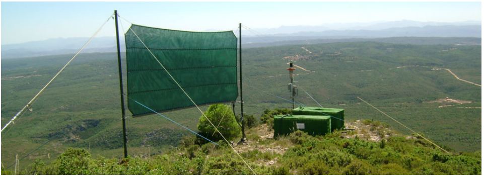
Figure 1.25: Picture of a fog collector made of meshes. The structure is vertical, allowing the wind to blow through it. The water droplets transported by the wind may collide with the mesh and drain towards a gutter below the net. From [131].
