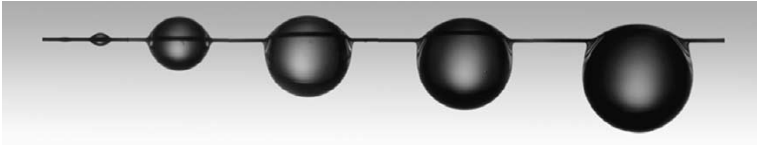
Figure 1.10: Pictures of silicone oil droplets on a horizontal fiber whose radius is r = 12 \mu\text{m} . From left to right the volume of the droplet increases \Omega = 0.01, 0.10, 0.23, 0.32 and 0.52 \mu\text{l} . From [80].
