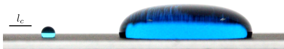
Figure 1.6: Picture of two blue-dyed water droplets on a hydrophobic solid surface (credit: J. Van Hulle). (left) A small volume, \Omega = 3 \mu\text{l} , adopts a spherical shape ( \text{Bo} < 1 ). (right) A larger volume, \Omega = 500 \mu\text{l} , adopts a puddle-like shape ( \text{Bo} > 1 ).
