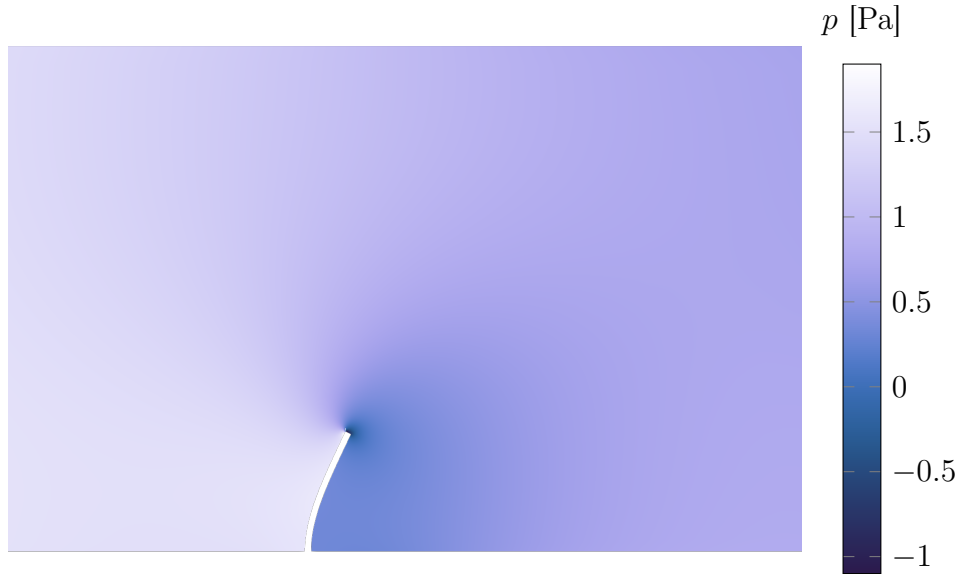
Figure 3.4: Flow field around cantilever beam in crossflow using SU2
