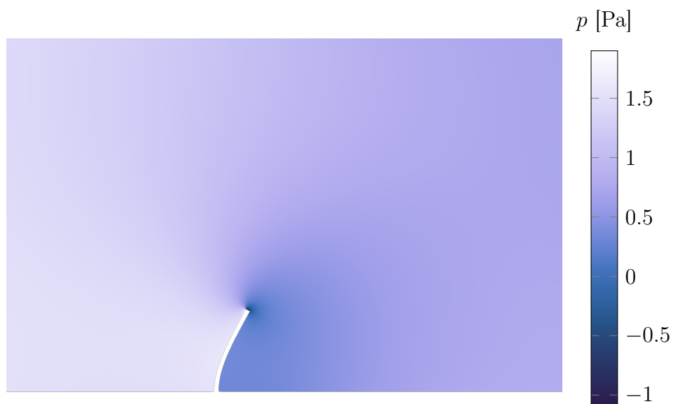
Figure 3.8: Flow field around cantilever beam in crossflow using SU2 and pyBeam
