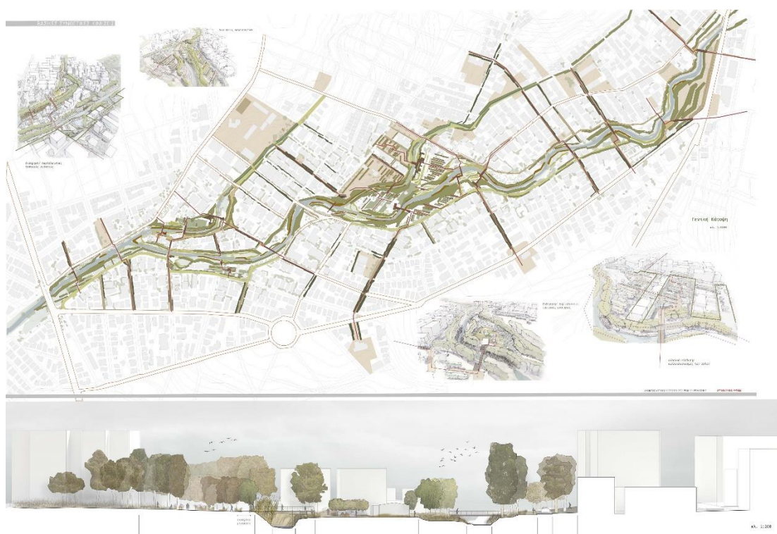
Figure 2. Exemplary intervention at the stream of Pikrodaphni: conceptual plan (upper part), and correlation of the zone of the stream with a green urban plantation zone (lower part).
