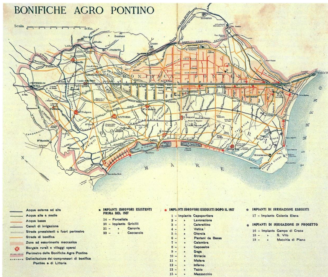
Figure 4. ONC, General map of the Pontine Plain showing canals for external and high waters and low waters, drainage and irrigation systems, new towns and villages, December 1934. [21]
