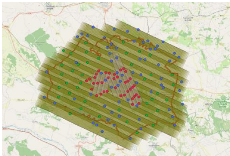
Figure 3. Detail of the aerial photogrammetry mosaic with indication of the Photographic Points of Support, denser in the central area
