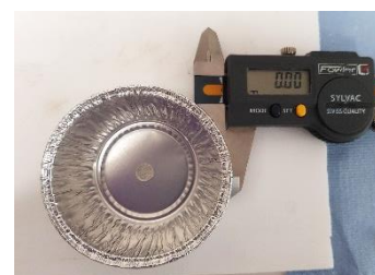
Figure S9: Variation of the swelling index and the linear swelling ratio as a function of time for PHU networks obtained from TMPTC-EDR148 formulations cured for 8h at 50°C with (A,B) no additives (dry) and (B,C) 5 wt% of water. Samples were first dried for 16h at 50°C under vacuum before swelling. Picture represents the measurement of swollen sample diameter with a caliper.
