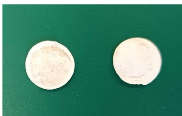
Figure IV-16: Separators after 40 cycles at 0.1 A g -1 of V 2 O 5 /CNT (left) and V 2 O 5 /PDA/CNT (right) electrodes.
