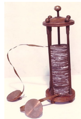
Figure I-1: Voltaic pile built in 1800 1 .
