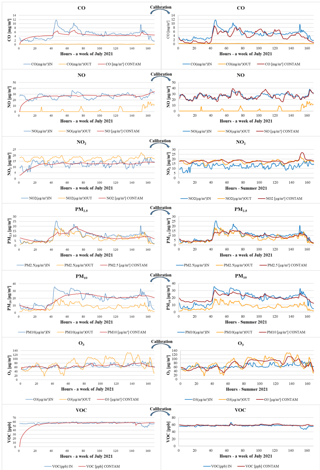
Fig 5.2. Hourly concentration of indoor and outdoor measurements and indoor results by CONTAM (168 hours = 7 days; 18-24 July 2021) – Case study house, a) Average emission rates b) Calibrated emission rates.
