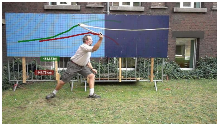
Fig. 7 Photo and plot of hook and hand trajectories from the beginning of the elliptical phase to the end. The concave flexion of the dart can be seen when the spear-thrower is in its ascending phase.
