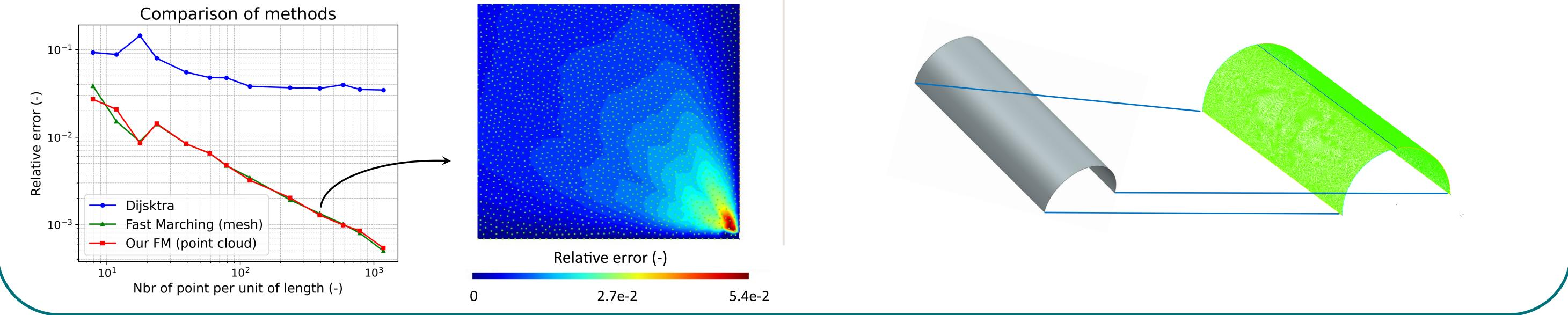
An algorithm to **match the geometry** between the model (blueprint or 3D) and the 3D scan.
