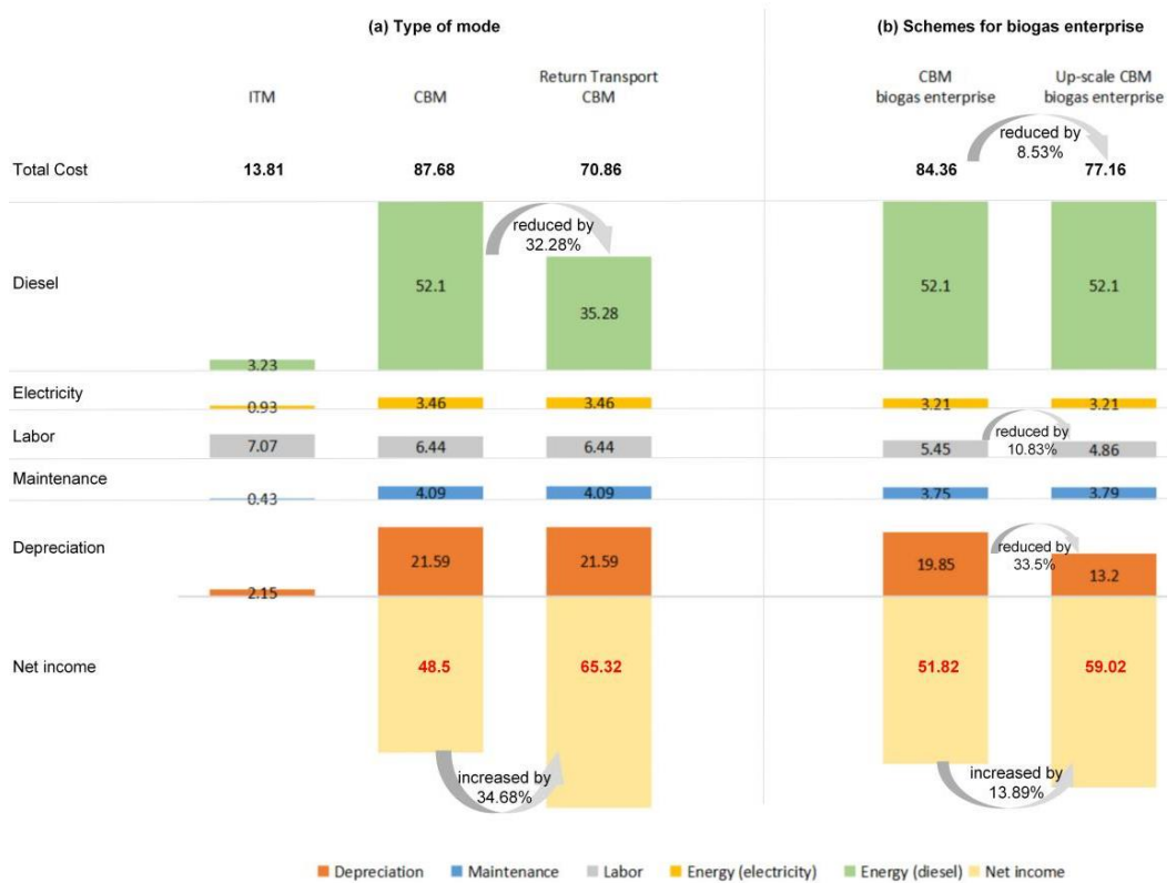
Figure 5-6. Economic viability analysis including economic costs and net incomes based on per function unit. (a) Comparisons between MSM modes (ITM, CBM and CBM traffic optimization scenario). (b) Based on the perspective of biogas enterprise of CBM, the original operation pattern and up-scale scenario were contrasted. Black numbers indicate the operating expenses of subitems. Bolded indicate total cost, red is net income. The major changes are represented by gray arrow.
