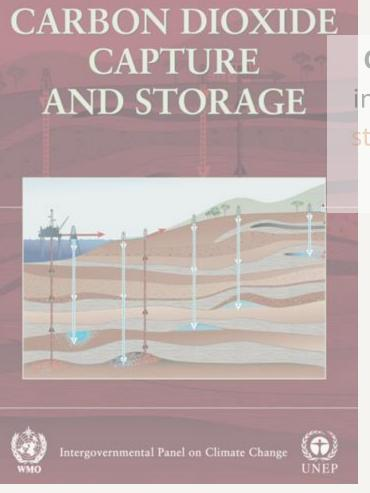
**CCS** = "the process of *separating CO2 from emission sources* in industrial or related energy sectors, transporting it, and securely storing it in geological formations, isolated from the atmosphere for the long term" (IPCC, 2005).
