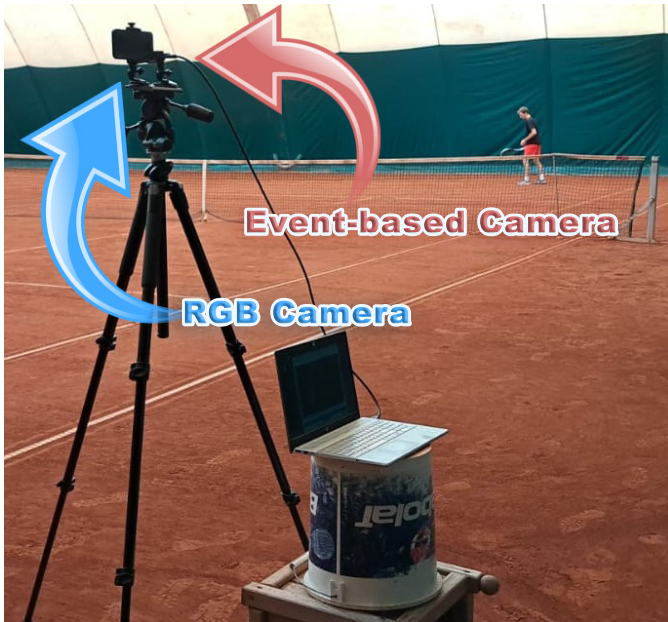
Fig. 2. Camera setup. Picture of our bi-camera setup used for sports data collection. We align both the RGB camera and event-based camera on a tripod.
