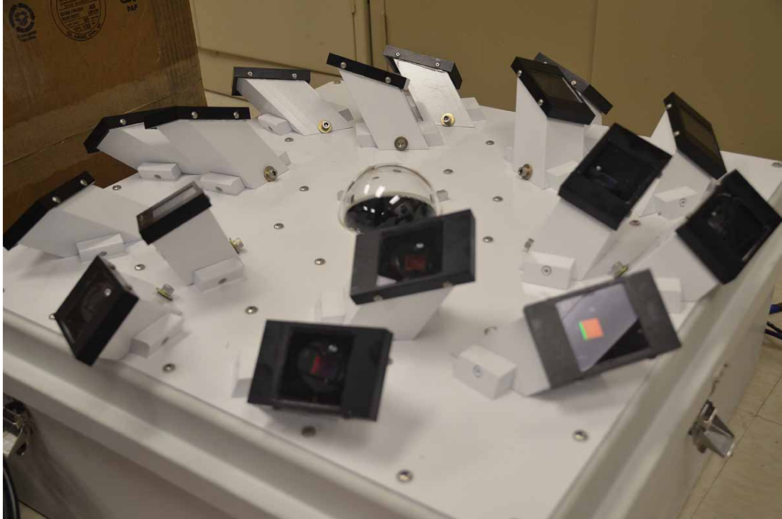
Figure 4A – The CAMS Spectrograph (CAMSS), consisting of 16 spectrographic cameras that operate in conjunction with the CAMS California meteor triangulation network.
