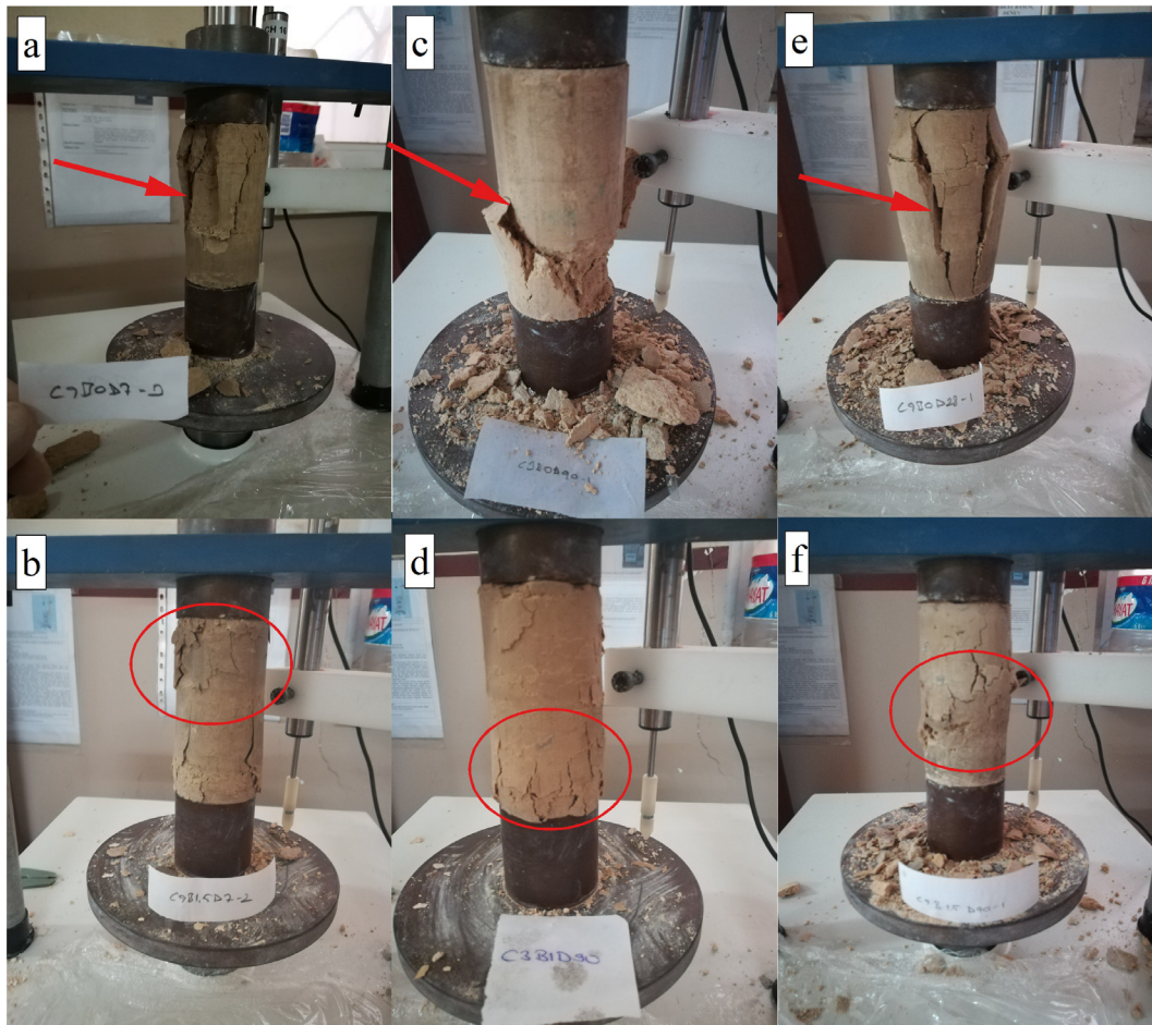
Fig. 10. Image of fracture patterns of specimens a) 9% cement treated (C9B0D7) b) 9% cement treated with 1.5% PBS content (C9B1.5D7) c) 3% cement treated (C3B0D90) d) 3% cement treated with 1.0% PBS content (C3B1.0D90) e) 9% cement treated (C9B0D28) f) 9% cement treated with 1.5% PBS content (C9B1.5D90).
