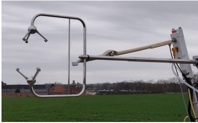
Figure 1.10: Example of an eddy covariance system configuration with a three-directional sonic anemometer (Gill HS-50) and a closed-path infra-red gas analyzer (LICOR 7200). Photo taken in BE-Lon.
