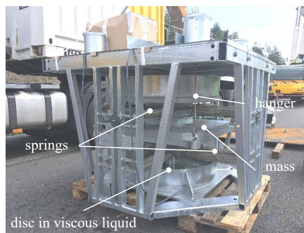
Figure 4. Tuned mass damper
