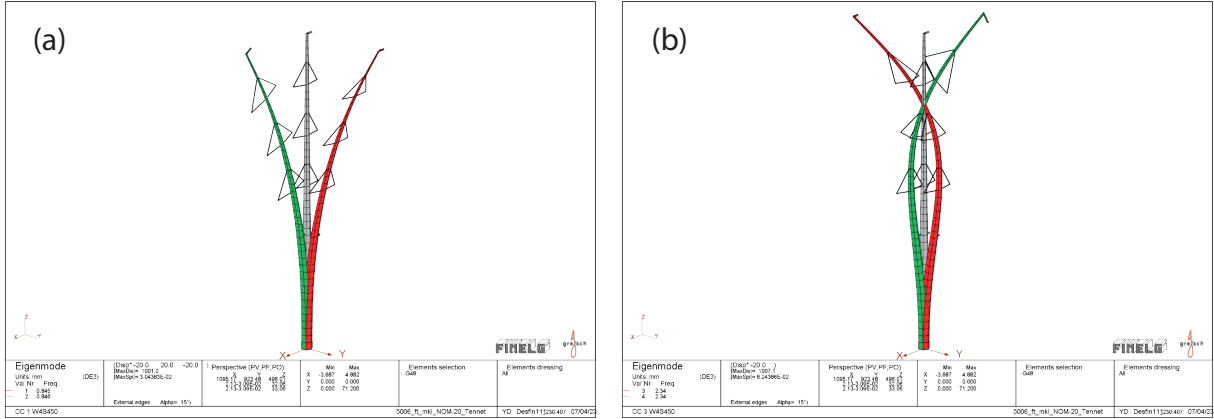
Figure 2. Mode shapes: (a) mode 1 (red), mode 2 (green); (b) mode 3 (green), mode 4 (red).
