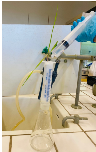
A. Customised device for root-exudate extraction
