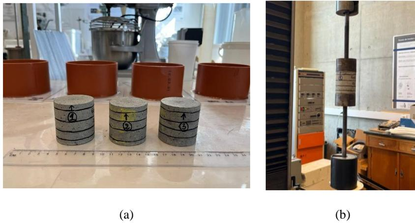
Fig. 4—Cored of printed samples (a) and the INSTRON instrument using for tensile strength test (b)
