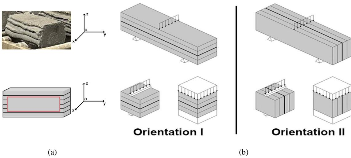
Fig. 3—Schematic depicting the printed sample and the illustration of the sampling (a), along with the various orientations of load application on the samples [9] (b)
