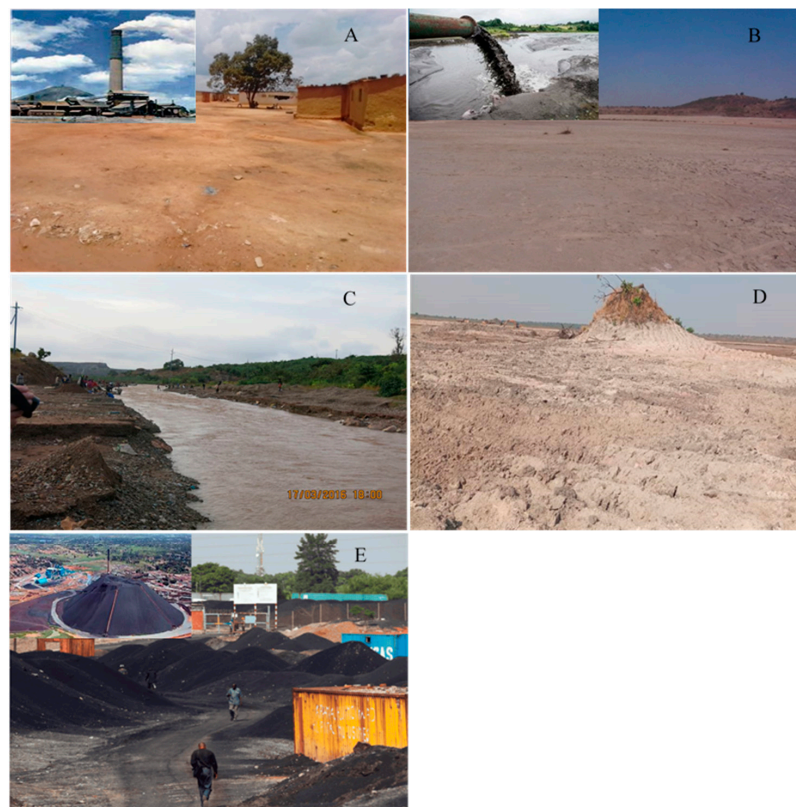
Figure 2. Main types of mine tailings, and contaminated soils and sediments in the KCB. (A) Soil contaminated by emissions from the smelter, (B) wastes from concentrates of Cu and Zn sulfides by
