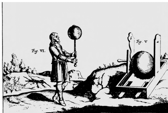
Figure 5: Otto Von Guericke holding a sulphur globe he charged by rubbing and used to test the interaction with different objects. Objects were initially attracted by the globe but then repelled if they touched it. Taken from [6].
