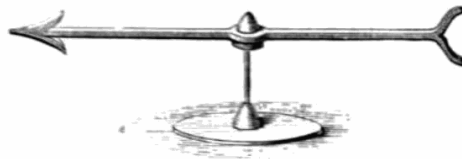
Figure 4: The versorium , William Gilbert's instrument used to test the attraction and repulsion of objects charged by friction. By electrostatic induction, the metallic needle points to a charged object. Taken from [5].
