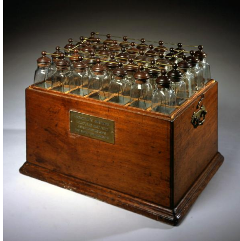
Figure 7: The first electric battery invented by Benjamin Franklin who connected multiple Leyden jars together to increase the amount of electricity stored. Illustration from benfranklin300.org .
