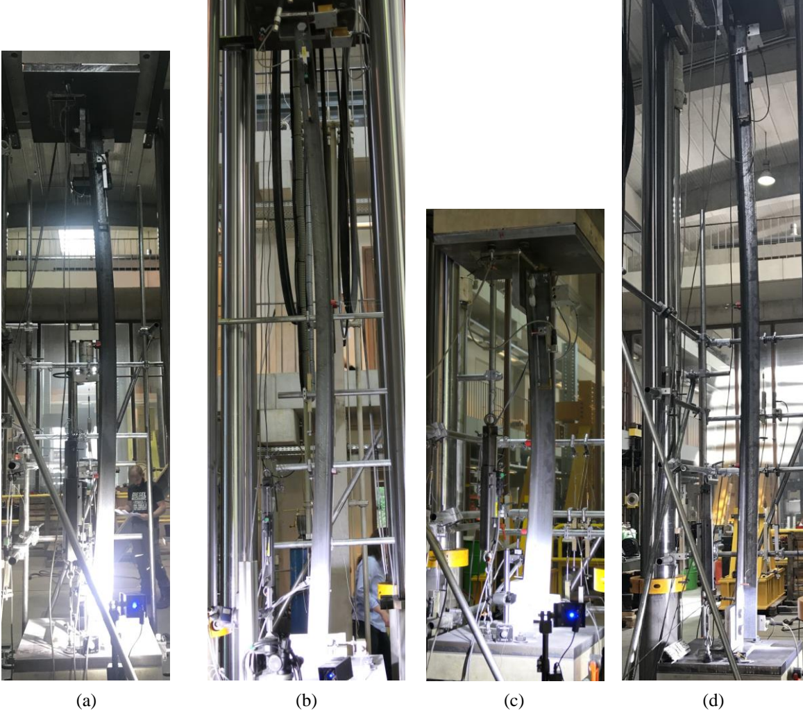
Fig. 6. Pictures at collapse of the two longest specimens with 1-bolt end joints (a:S13, b:S14) and of the shortest (c:S21) and the longest (d:S23) specimens with 2-bolts end joints
