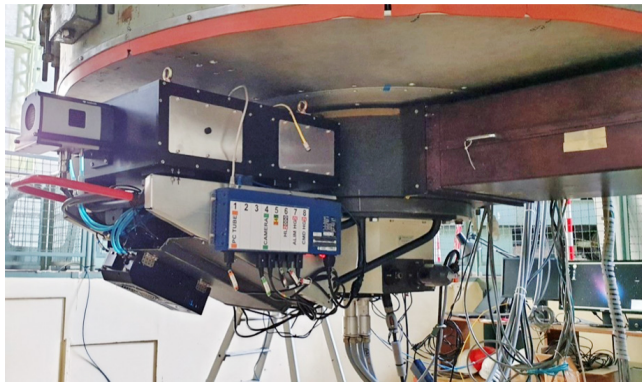
Fig. 1. MISTRAL (to the left of the image) installed at the folded Cassegrain focus of the 1.93 m telescope at OHP.
