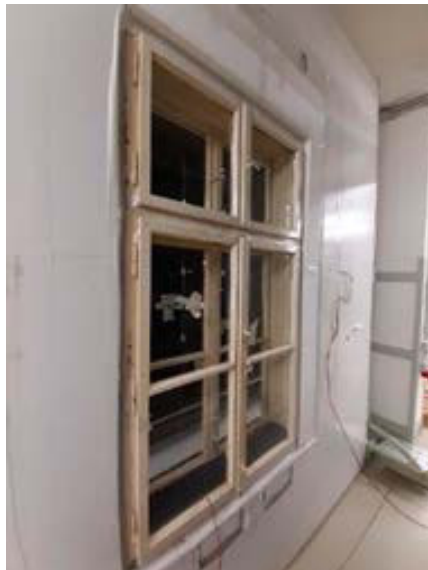
Figure 1: Historic double window (end 19 th century) in the test stand of the of the Municipal Department 39, Vienna, window taken from the stock of the convent Mauerbach, photo Peter Hunger.
