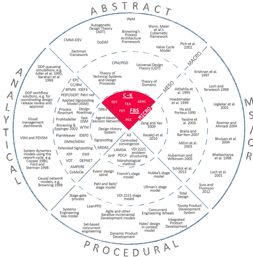
Figure 2.5: Classification of design process models, highlighting those of particular interest within the micro and abstract dimensions (Wynn and Clarkson, 2018).
