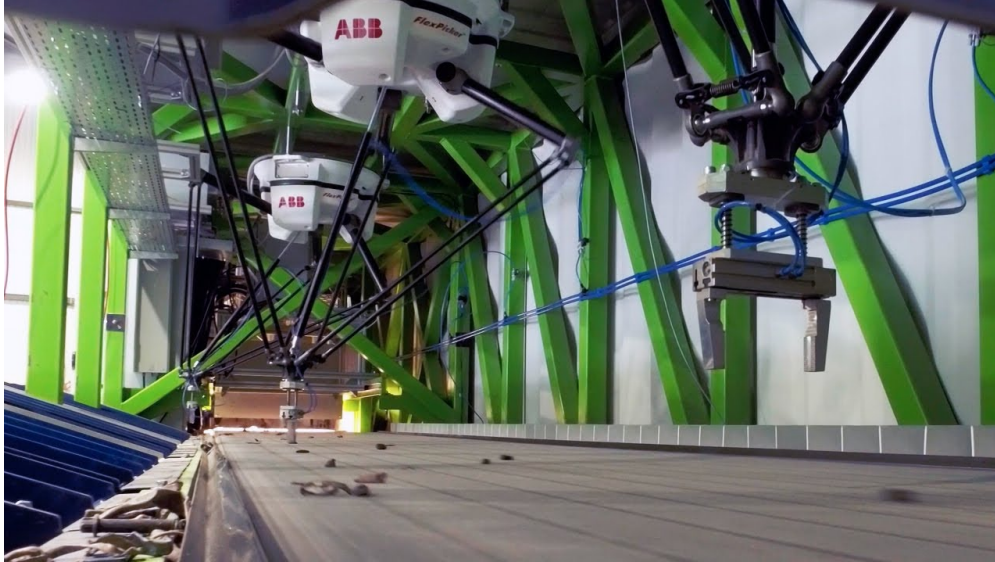
Figure 1: Photo of the PICKIT project at the GeMMe (Georesources, Mineral Engineering & Extractive Metallurgy) lab with a focus on the ABB IRB 360 Flexpicker robots sorting scrap metal.
