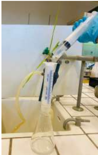
A. Customised device for root-exudate extraction
