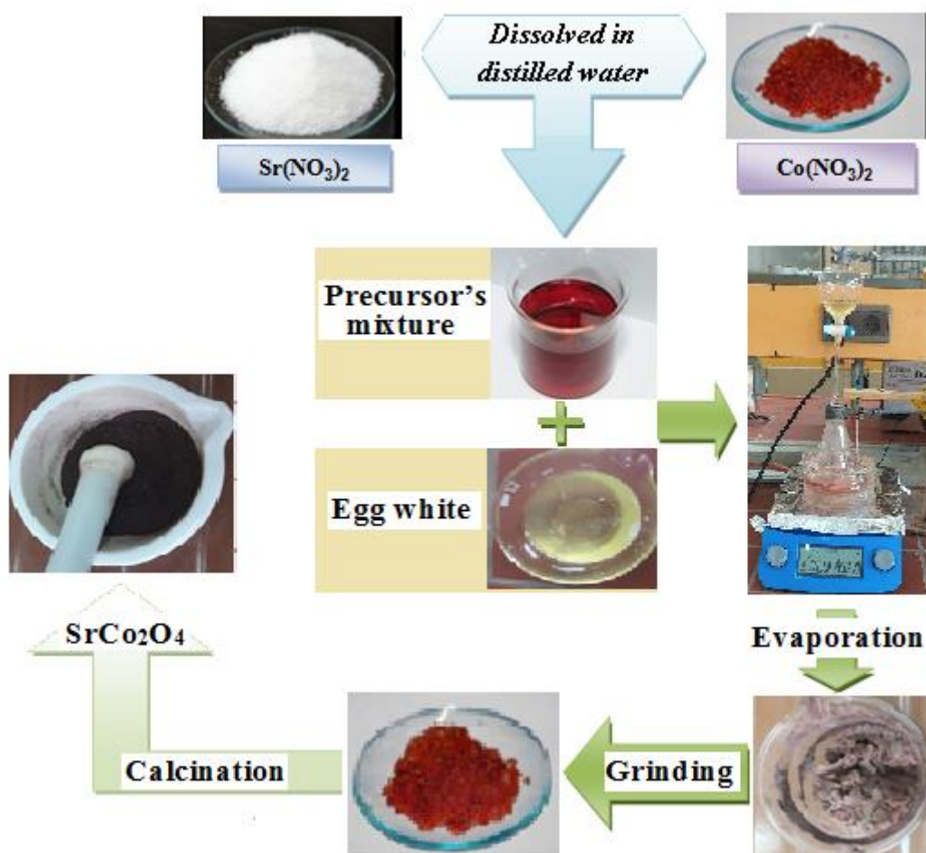
Fig. 1. The preparation steps of \text{SrCo}_2\text{O}_4 nanoparticles.
