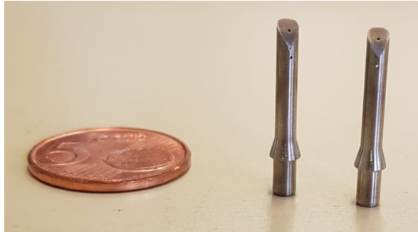
Figure 2.34: Heads of virtual four-hole probe to be installed with pneumatic lines and fast-response sensors.
