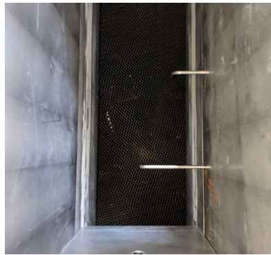
Figure 2.21: Location of the pitot tubes upstream of the test section.
