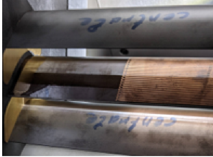
Figure 2.48: Surface-mounted hot-film sensors on the blade surface.
