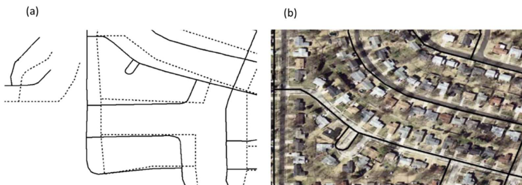
Figure 11: Representation of (a) vectorial model (b) raster model, from the same area of visualization and analyzed. Adapted from the book Encyclopedia of GIS.
