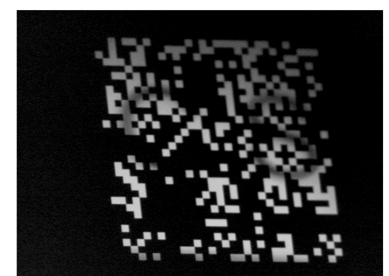
Same image with a 32x32 mask applied on the DMD
