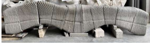
Figure 3- Printed segment assembled as a bench in the framework of CIRMAP project [16]
