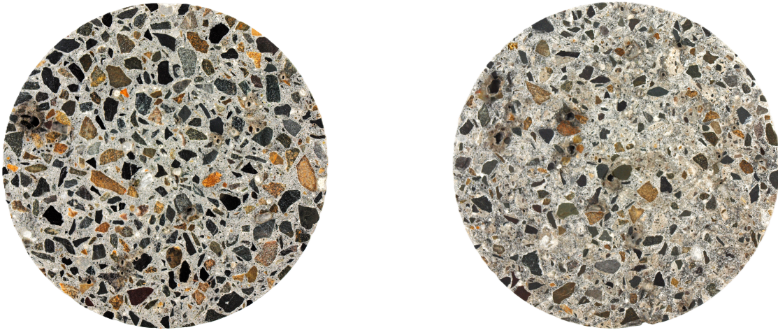
Figure 1.4: Pictures of a Natural Aggregates Concrete (NAC, left) and Recycled Aggregates Concrete (RAC, right) produced for this research.
