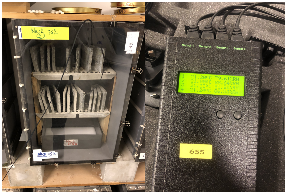
Figure 4.3: Left: Chambers used for the static sorption and desorption experiment, with the RH and temperature probe and the samples inside. Right: sensor housing displaying the measures for the four probes used.
