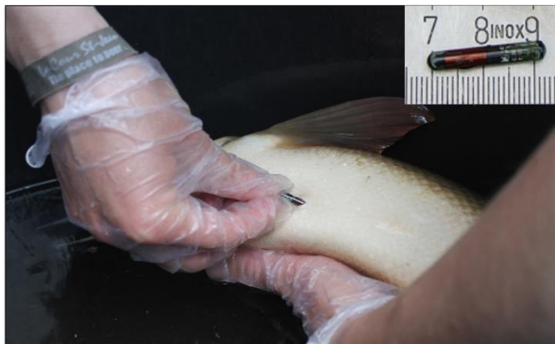
Figure 2 : Transpondeur RFID (Texas Instrument)
