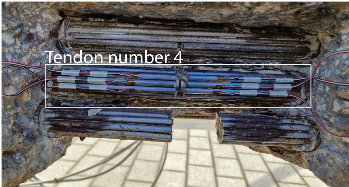
FIGURE 5.13: Damaged scenario 4 with tendon number 4 half cut.
