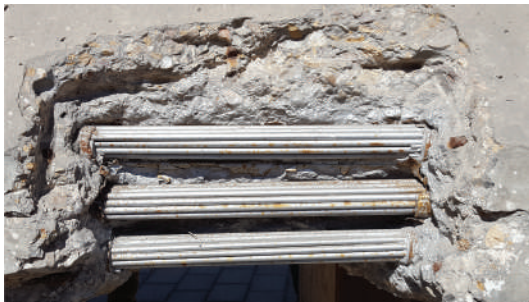
FIGURE 5.3: (a) Representation of the beam with the shaker, the trolley and the damaged section, (b) picture of the experimental setup during the tests, (c) tendons and damaged section and (d) the portable circular saw.
