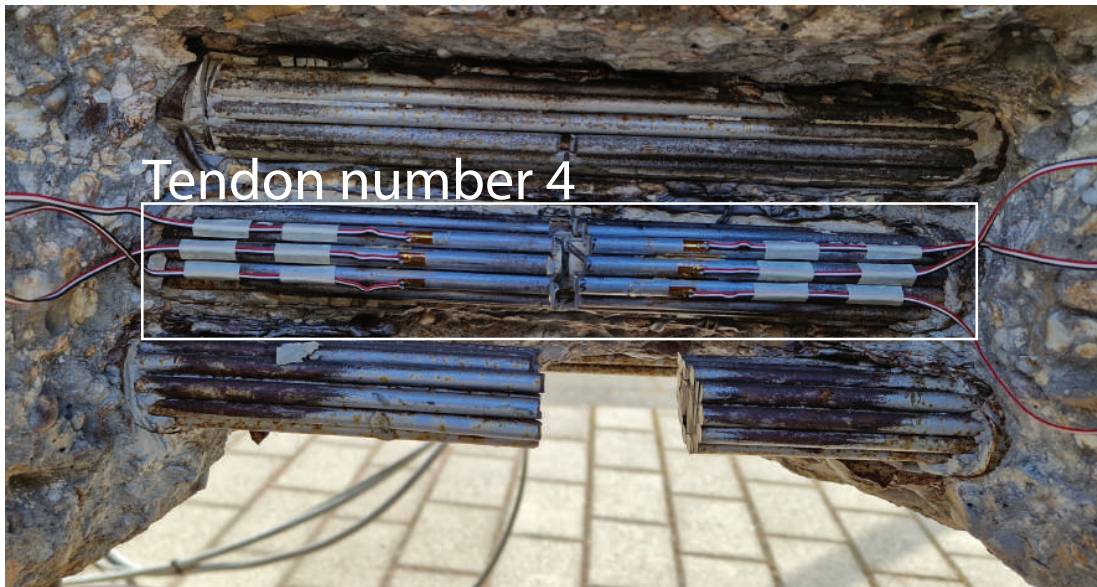
FIGURE 5.13: Damaged scenario 4 with tendon number 4 half cut.
