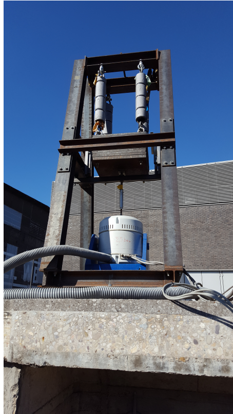
FIGURE 5.6: Picture of shaker on the beam.
