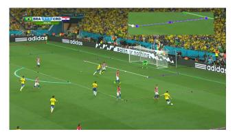
Figure 3. Illustration of annotations on a SoccerNet-v3 [6] image as used for the camera calibration challenge. As shown in the zoomed snapshot, annotations consist of points and the labels of the objects they belong to.
