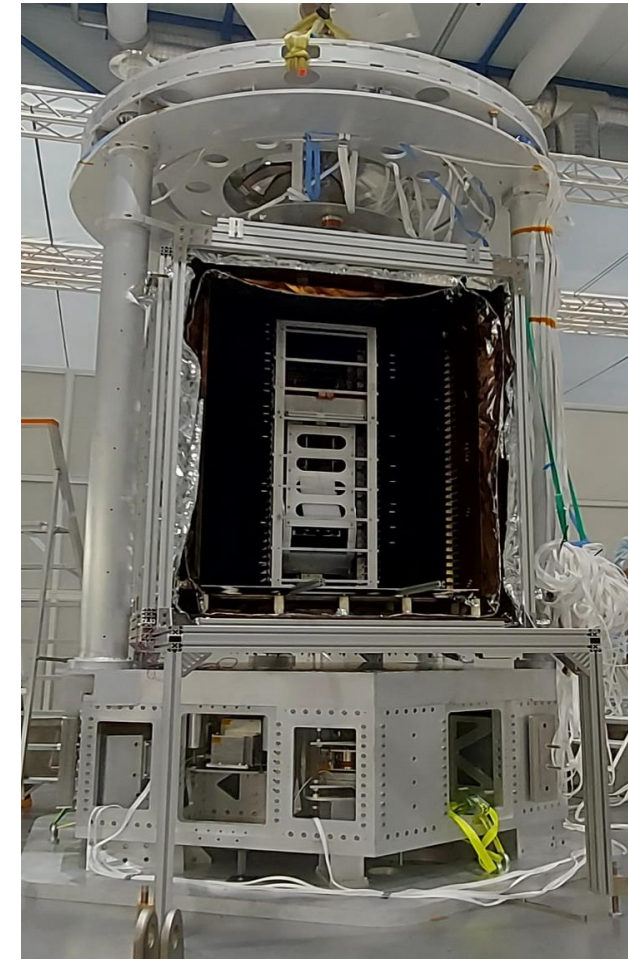
After integration of outer cryostat including LN 2 shield and GHe panels
