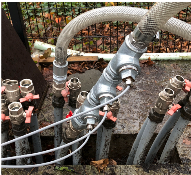
Fig. 3. T-shaped pipe tool ensuring the watertightness of the system and an alteration as limited as possible of the fluid flow within the U-shaped pipe.
