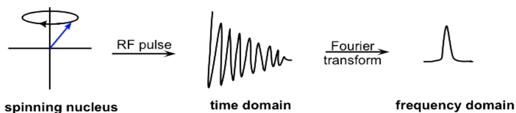
Figure 11 Simplified diagrams to illustrate NMR experiment ( https://kpu.pressbooks.pub/organicchemistry/chapter/6-5-the-nmr-theory/ )
