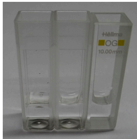
Figure 13. Water to cuvette meniscus for a new PMMA cuvette (left), cleaned PMMA cuvette (middle) and optical glass cuvette (right).
