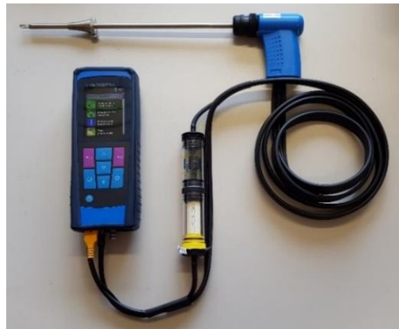
Figure 106. 'Multilyzer STx' combustion analyser portable meter.
