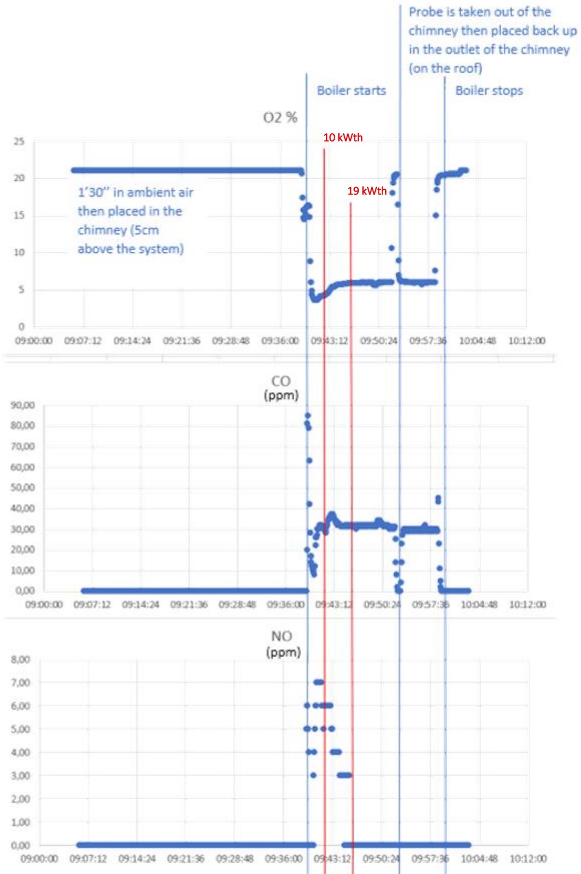
Figure 95. Field-test pollutant emissions in Huy - boiler only (part 2/3).
