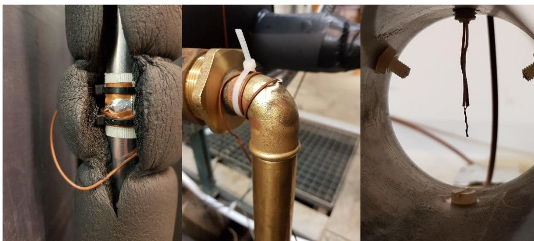
Figure 77. Thermocouples assembly configurations: surface, elbow and air thermocouples (in the system's chimney).
