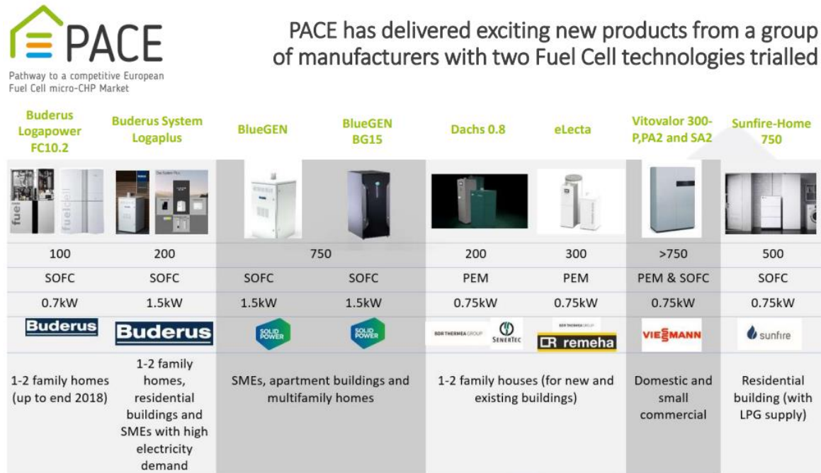
Figure 22. Fuel cell micro-CHP systems commercially available in Europe. The reported power output is the nominal electrical power output; the previous numeric row corresponds to the amount of units installed in Europe through the PACE supporting program. Reproduced slide from the Final Conference of the PACE European Union project (26 April 2023) [393], that aimed to demonstrate through field-test installations and monitoring in real applications the capability of fuel cell products to reach a commercial mass market [347].
