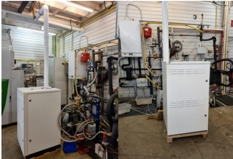
Figure 105. Tested micro-CHP SOFC in the laboratory facilities of the University of Liege [447].
