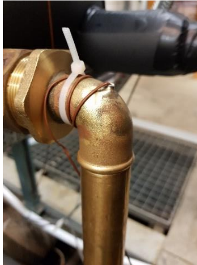
Figure 44. Thermocouple elbow immersion sleeve (without insulation features).
