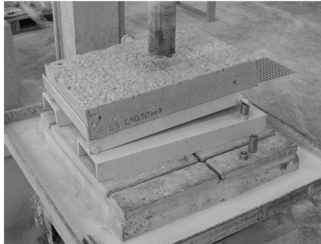
b) Slab positioning for coring at an angle of 4°
