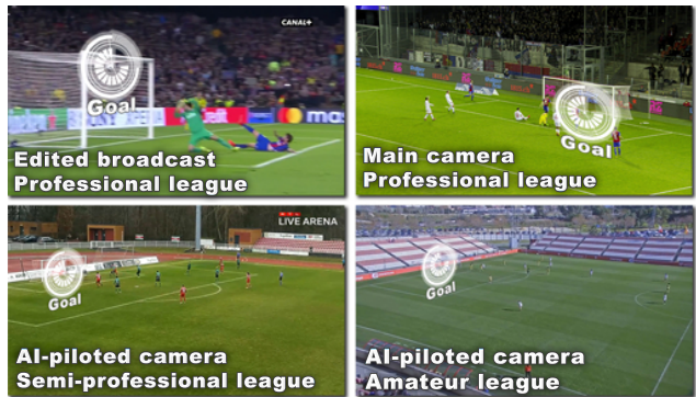
Figure 1. Domain gap between different leagues and broadcast quality. We showcase four domains: (1) professional league broadcast from the SoccerNet dataset, (2) professional league unedited main camera feeds from the Swiss Super League, (3) semi-professional league AI-piloted camera from the BGL Luxembourg National Division, and (4) amateur league AI-piloted camera from Sevilla. Our analysis shows that transferring action spotting models from professional broadcasts to amateur AI-piloted camera is challenging due to different recording and broadcast editing quality.
