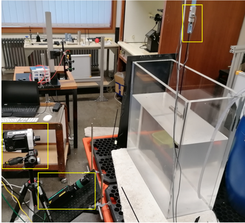
Figure 5.30: Picture of the first experimental setup. Three instruments are shown on this picture, and are framed by yellow rectangles. On the top right, there is the force sensor; on the lower left, there are the high speed camera and the laser used for PIV. Courtesy of S. Dorbolo.
